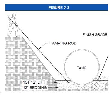
rods are recommended for free-flowing gravel and coarse sand.
